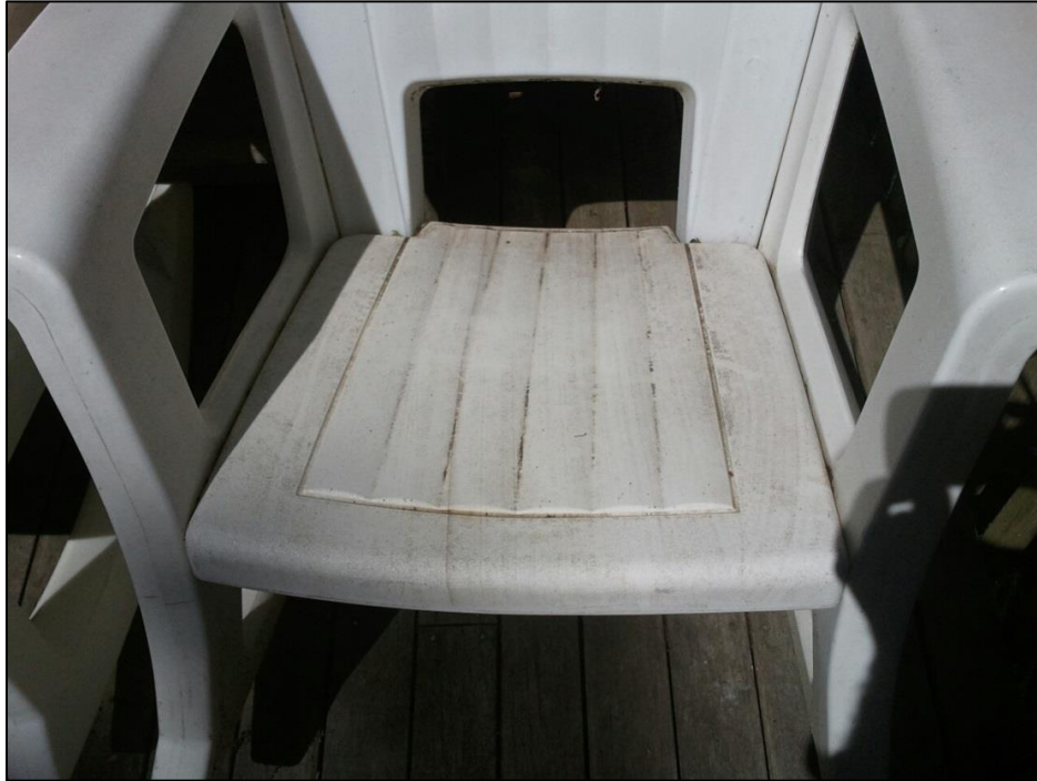
Cleaned with EcoSeal Citra-solve , left untreated over winter After 2 years, dry wiped before photo
