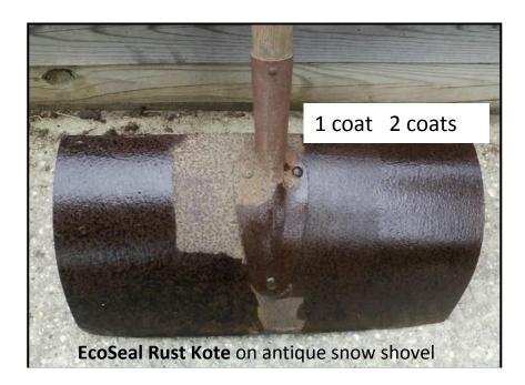
**Reaction and Cure Time:** Normal initial cure time is between 2 to 4 hours depending on the air temperature. Coated surface may be painted after 24 hour complete cure.
